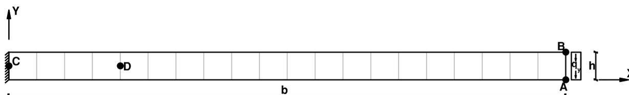
Figure 10: Typical mesh used for Abaqus discretization. Cantilever plate under uniform shear load.
