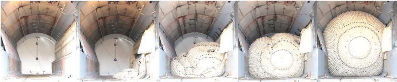
FIGURE 5 Sequence of deployment and initial air inflation for Test 6-AW.
