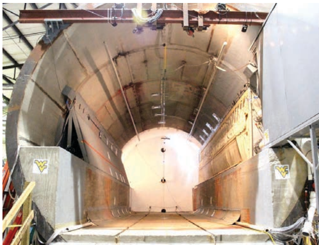
FIGURE 2 Tunnel section and folded plug placed in tunnel sidewall before beginning of test.
