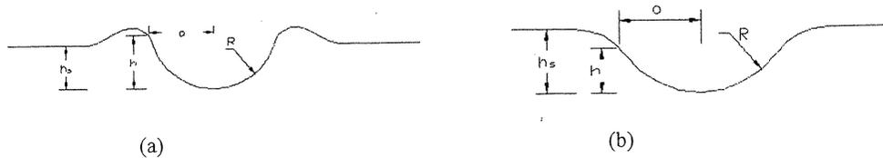
FIG. 6. (a) piling-up mode (b) sinking-in mode.
