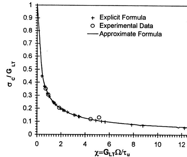
Figure 8. Nondimensional compression strength as a function of the nondimensional number.
