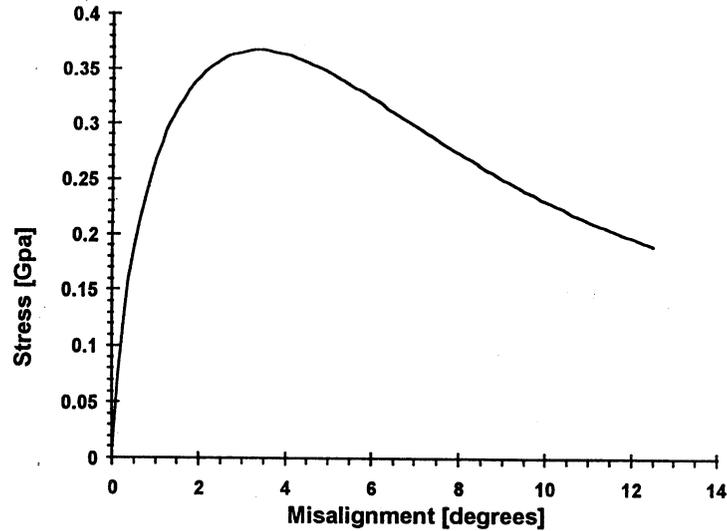
Figure 5. Applied stress  $\bar{\sigma}$  as a function of misalignment. Loading of the sample proceeds from left to right, until compression failure at the apex of the plot.
