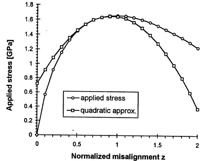
Figure 7. Comparison of the applied stress  $\bar{\sigma}$  [Equation (22)] and a truncated polynomial expansion, for AS4/E7K8.
