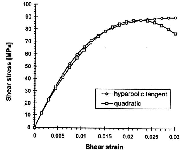
Figure 6. Fit of the hyperbolic tangent with a quadratic polynomial.
