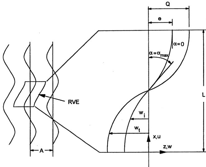
Figure 2. Representative Volume Element and variables used.
