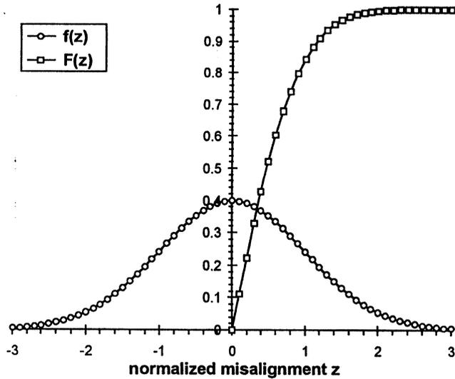
Figure 1. Standard probability density function  $f(z)$ , and  $F(z)$  vs. the normalized misalignment angle  $z$ .
