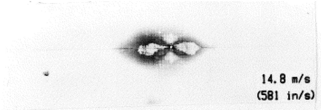
Figure 3.1:  $[0_3/90_3/0_3/90_3/0_3]$  specimen after impact at 14.8 m/s velocity with a 2.22 cm (46 g) diameter ball and 5 J impact energy. The x-ray image shows significant delamination [7].
