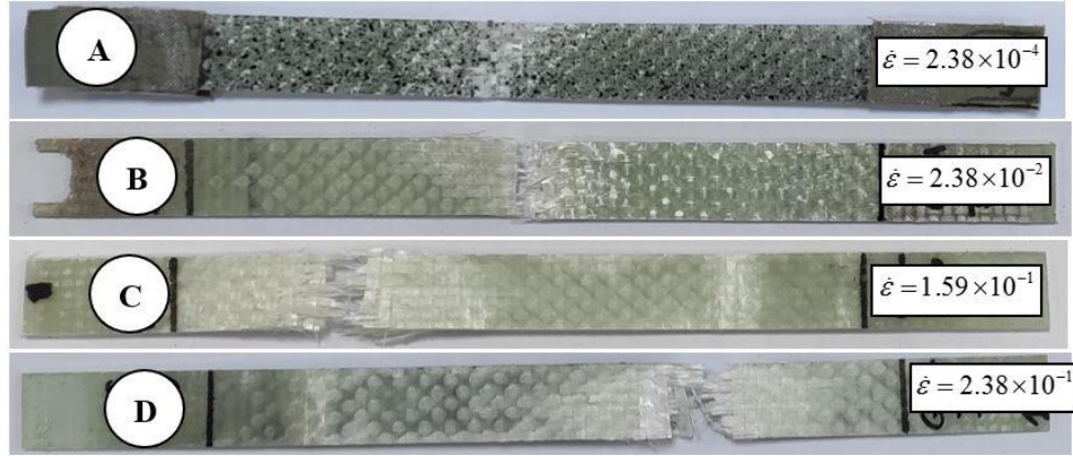
Fig. 24. Failed specimen of different tensile strain rates
