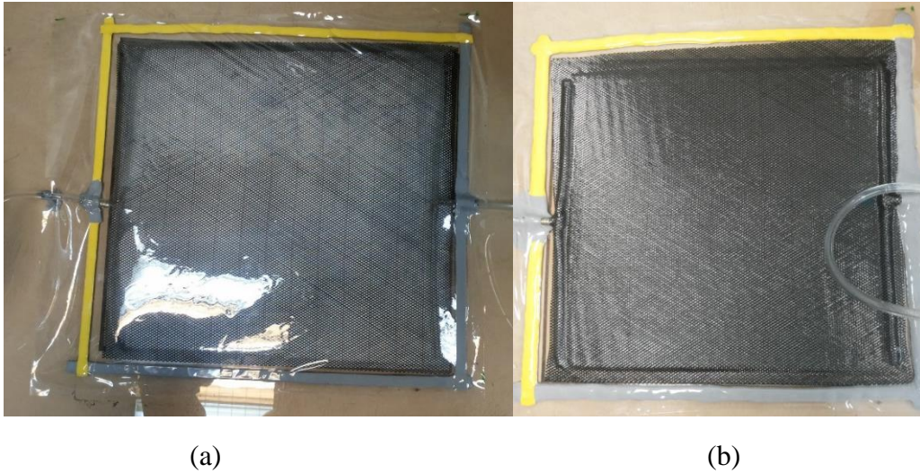
Fig. 6. Photograph of the vacuum infusion process of WF laminate with black mesh
