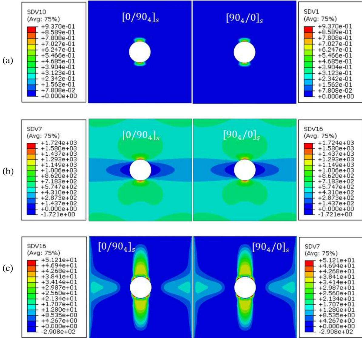
Fig. 10. Comparison between  $[0/90_4]_s$  and  $[90_4/0]_s$  laminates. a) Crack-density evolution on 90° plies b) Longitudinal stress on 0° plies and c) Longitudinal stress on 90° plies.
