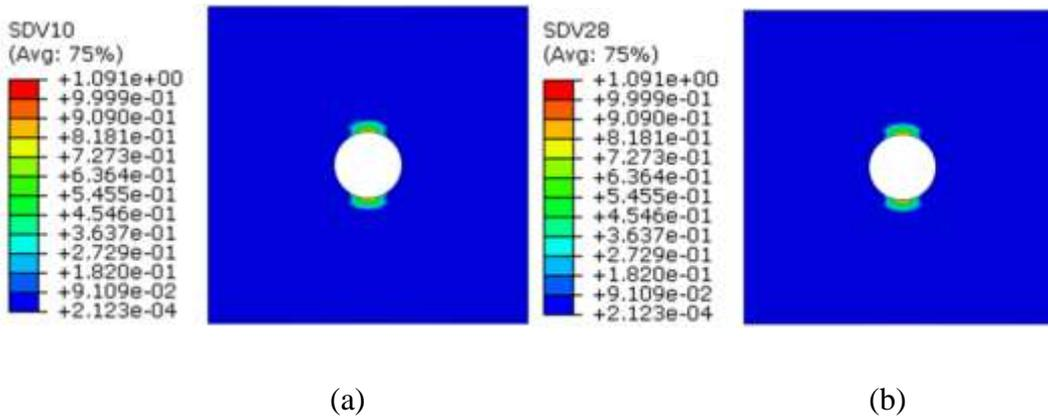
Fig. 7. Crack-density evolution in [0/90<sub>7</sub>/0]<sub>2s</sub> laminate. a) 90° external cluster, b) 90° internal cluster.
