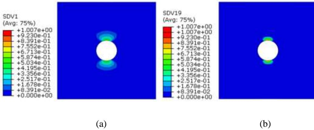
Fig. 6. Crack-density evolution in [90<sub>7</sub>/0]<sub>2s</sub> laminate. a) 90° external cluster, b) 90° internal cluster.
