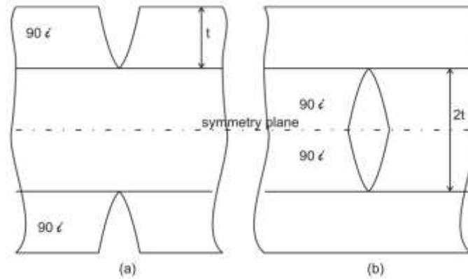
Fig. 8. Inverse laminates: a) crack in a surface 90° cluster, and b) crack in an interior 90° cluster.
