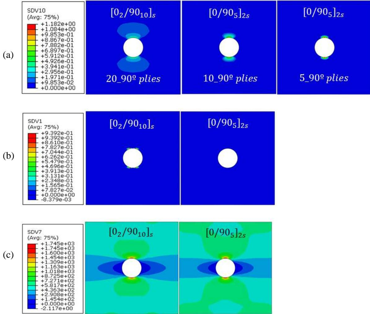
Fig. 3. Comparison between  $[0_2/90_{10}]_s$  and  $[90_5/0]_{2s}$  laminates. a) From left to right: 20, 10, and 5 ply, 90° clusters. Crack-density evolution on 90° plies, b) From left to right: 2 and 1 ply, 0° cluster. Crack-density evolution on 0° plies, c) Longitudinal stress on 0° plies and, d) Longitudinal stress on 90° plies.
