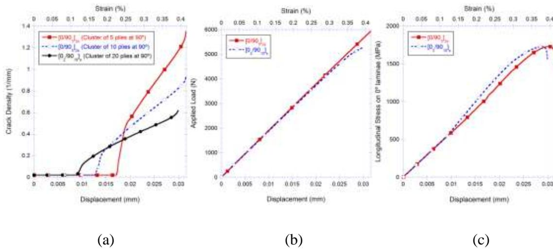
Fig. 2. Comparison of  $[0/90_5]_{2s}$  and  $[0_2/90_{10}]_s$  laminates: a) crack-density evolution on  $90^\circ$  plies in the node situated at the edge of the hole for three different clusters of  $90^\circ$  plies, b) Applied-load evolution and c) Longitudinal stress on  $0^\circ$  plies in the element situated above the edge of the hole.
