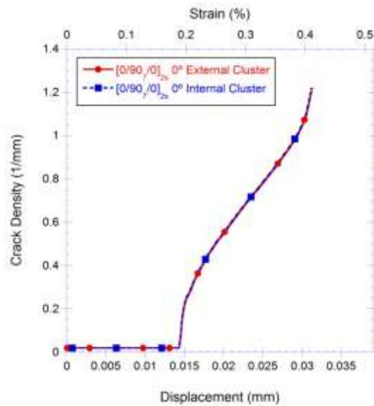
Fig. 5. Crack-density evolution on  $90^\circ$  plies in the node situated at the edge of the hole, for  $[0/90_7/0]_{2s}$  laminate
