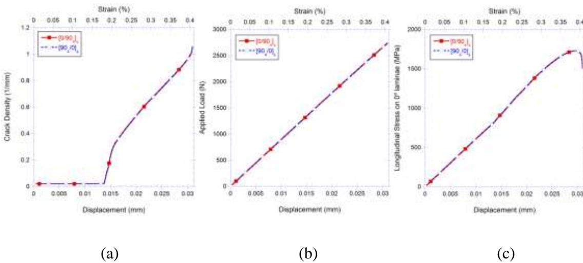
Fig. 9. a) Crack-density evolution on 90° plies in the node situated at the edge of the hole, b) Applied-load evolution of the laminate and c) Longitudinal stress on 0° plies in the element situated above the edge of the hole, for  $[0/90_4]_s$  vs  $[90_4/0]_s$  laminates.
