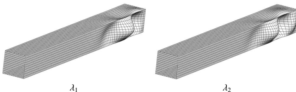
**Figure 3.** Clamped box under shear forces. Buckling modes corresponding to buckling loads  $\lambda_1$ ,  $\lambda_2$ .
