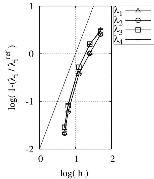
**Figure 2.** Clamped box under shear forces. Convergence of buckling loads with mesh refinement. The solid line represents  $h^2$  (for reference).
