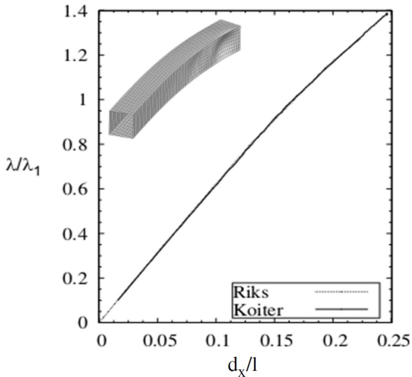
**Figure 4.** Clamped box under shear forces. Deformed configuration along the equilibrium path at  $\lambda = 52.20$  and equilibrium paths evaluated for both Koiter and Riks analyses. The graphed displacement  $d_x$  refers to the transversal displacement of point  $B$  (see Fig. 1).
