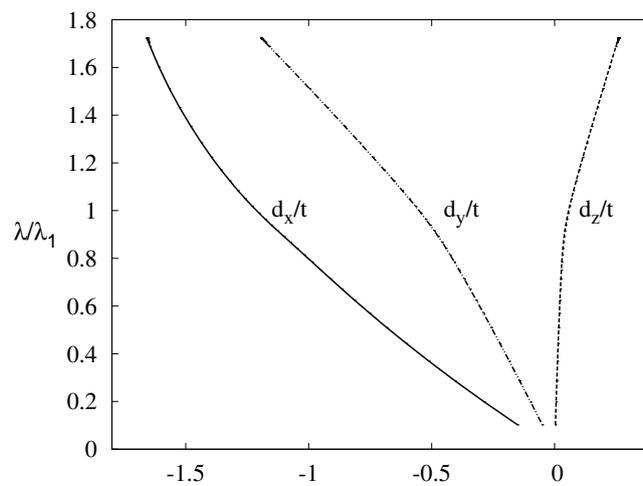
**Figure 5.** Clamped box under shear forces. Equilibrium path recovered using Koiter analysis. The graphed displacements  $d_x$ ,  $d_y$  and  $d_z$  refer to the displacements of point  $A$  (see Fig. 1).
