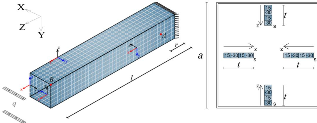
**Figure 1.** Geometry, boundary conditions, and load for clamped box subjected to shear load.
