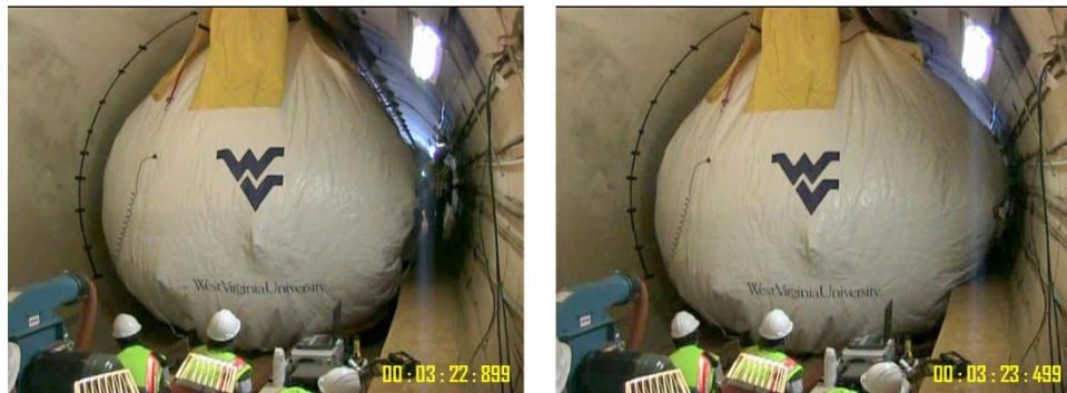
Figure 8: Release of the restraint during the inflation process
