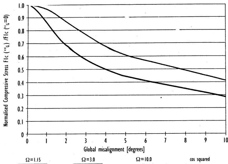
Figure 7: Normalised Compressive Strength versus Global Misalignment
