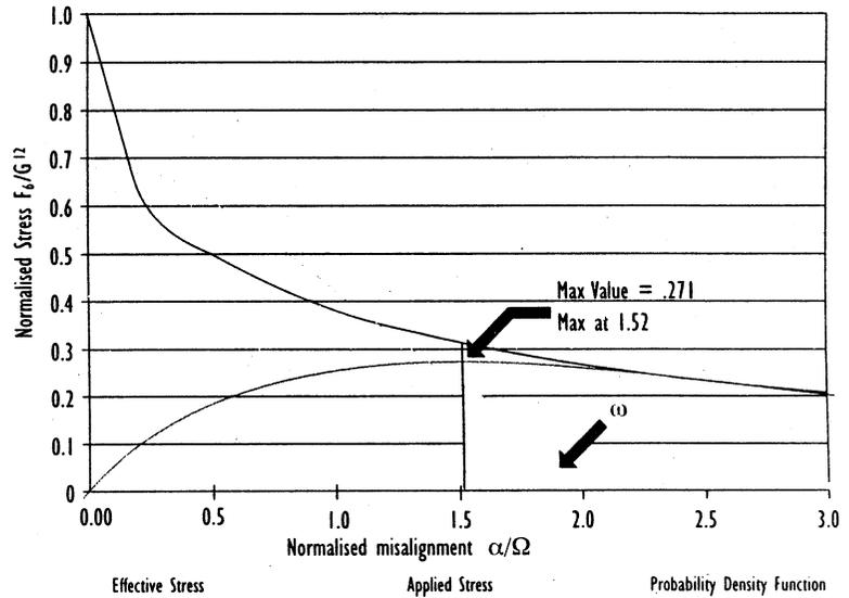
Figure 2: Combined Buckling/Misalignment Plot for 949/M30GC
