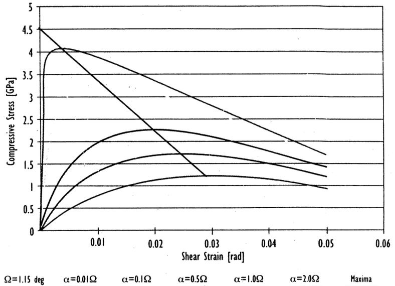
Figure 1: Bundle Stress versus Shear Strain in 949/M30GC
