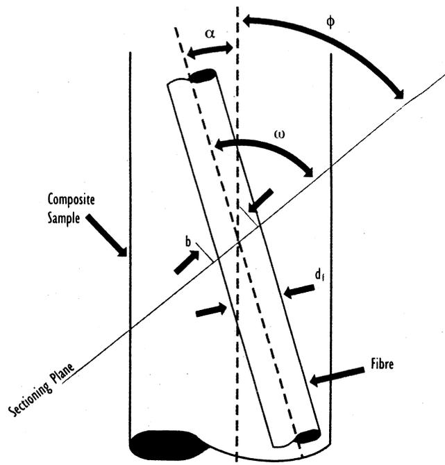
Figure 5: Misalignment Measurement Technique
