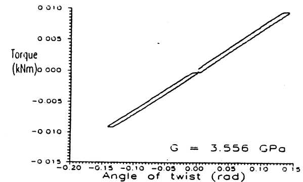
Figure 6. Torque vs. angle of twist curve for a torsion test.
