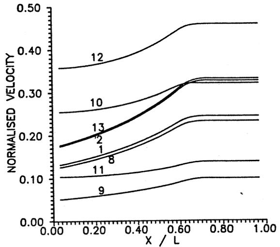
Fig. 10. Velocity distribution for tapered die, effect of variable permeability.
