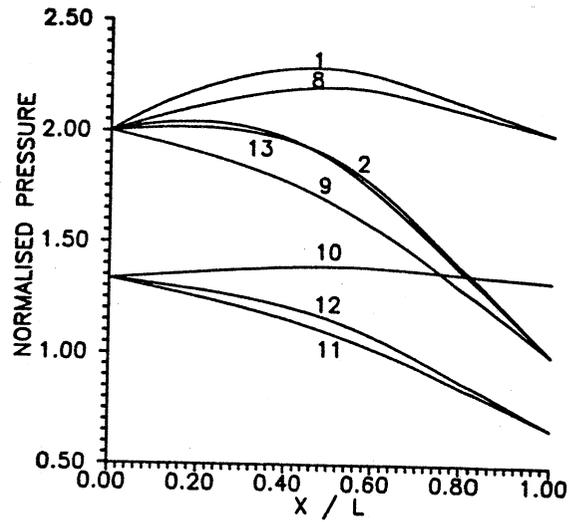
Fig. 9. Pressure distribution for tapered die, effect of variable permeability.
