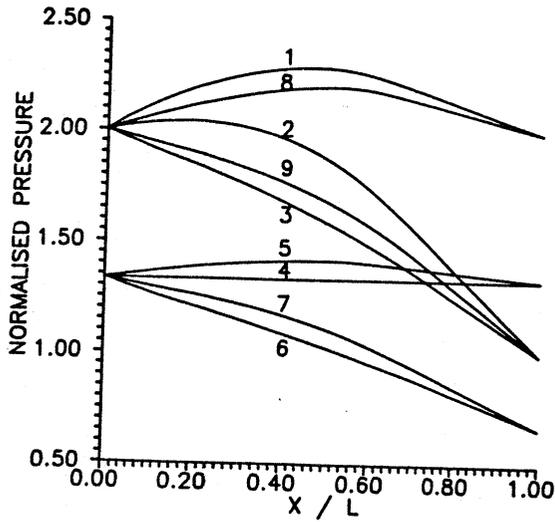
Fig. 7. Pressure distribution for tapered die, comparison with rectangular die.
