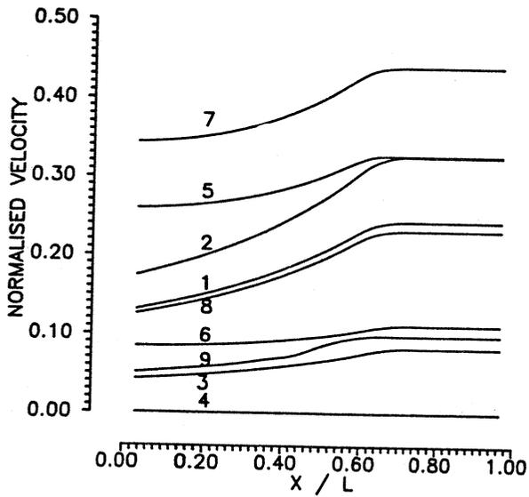
Fig. 8. Velocity distribution for tapered die, comparison with rectangular die.
