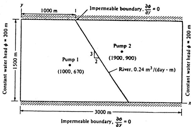
Fig. 1. Ground water flow<sup>4</sup> (Ex. 4.3)
